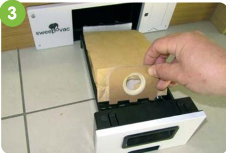
Replace the bag as shown **every 12 weeks (for normal domestic use)**. The bag can be changed at the appliance or the entire drawer can be carried to the bin and the bag disposed of there. Ensure the three cardboard lugs are slotted home. Push down clip to release the bag.
